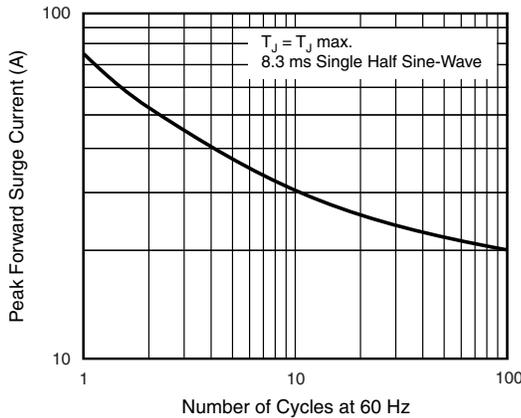
Fig. 5 - Maximum Non-Repetitive/Peak Forward Surge Current
