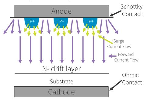
Our diodes feature the MPS (Merged PIN Schottky) design which is more robust and reliable than standard Schottky barrier diodes. MPS diodes also offer superior surge current capability, low leakage current and are less vulnerable to surface imperfections.
