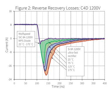
These graphs compare the reverse-recovery charge ( $Q_{rr}$ ) of 650V (figure 1) and 1200V (figure 2) SiC Schottky diodes and silicon bipolar diodes at various temperatures. The shaded areas represent the wasted energy due to the recombination of the minority carriers of the silicon bipolar diode.
