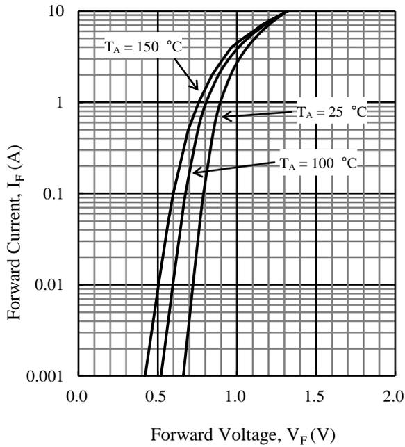
Figure 5.  $I_F - V_F$  Typical Characteristics
