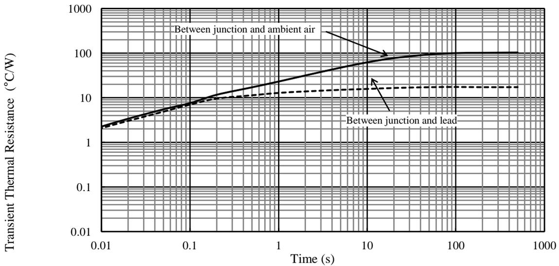
Figure 4. Typical Transient Thermal Resistance<sup>(6)</sup>
