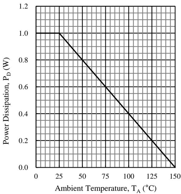
Figure 2. Power Dissipation Curve<sup>(4)</sup>
