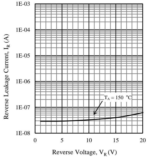
Figure 6.  $I_R - V_R$  Typical Characteristics<sup>(7)</sup>
