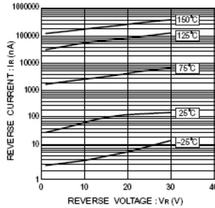
Fig.2 Reverse characteristics
