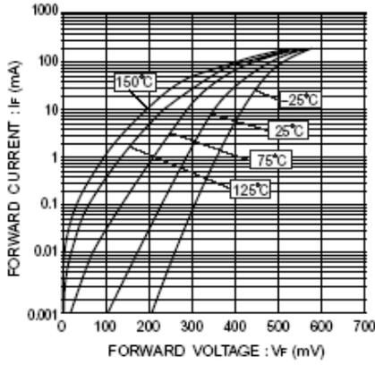
Fig.1 Forward characteristics
