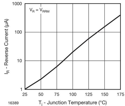
Fig. 4 - Max. Reverse Current vs. Junction Temperature
