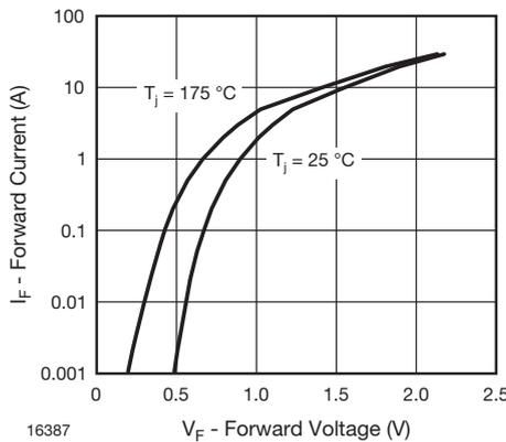
Fig. 2 - Max. Forward Current vs. Forward Voltage
