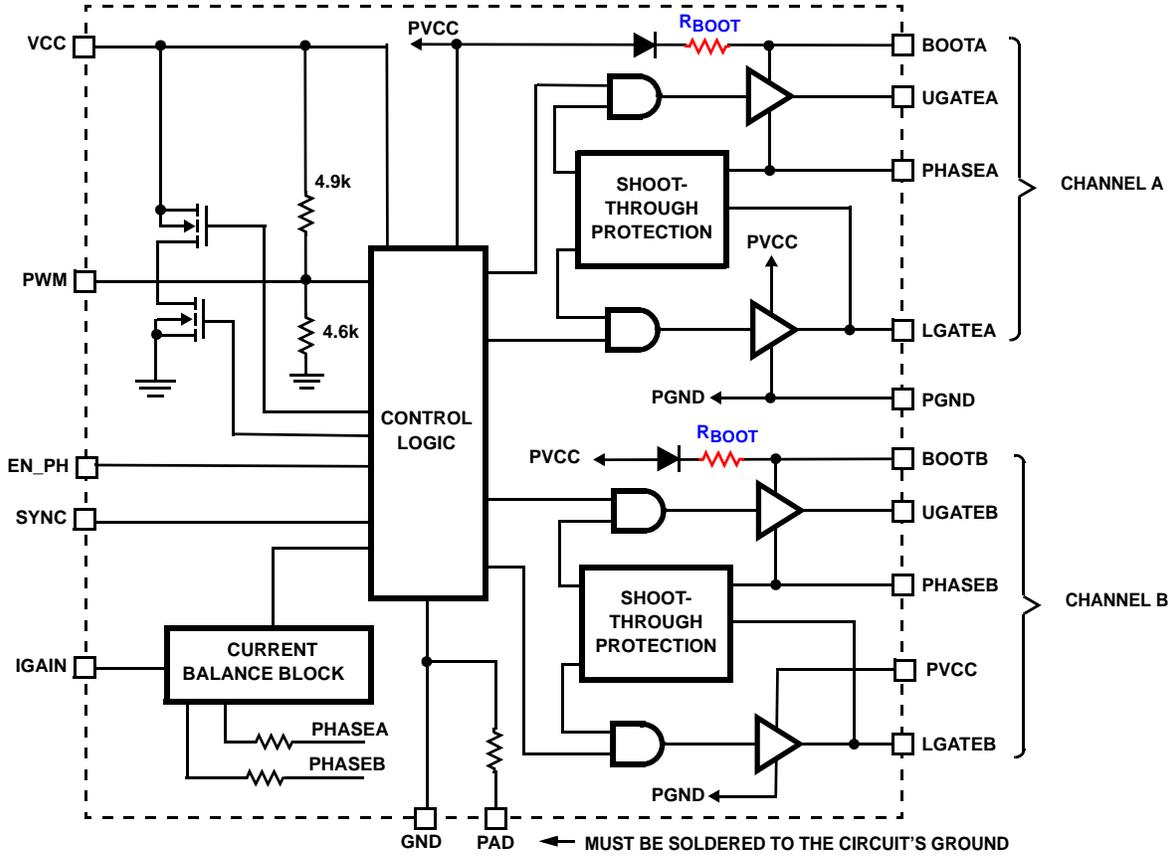
INTEGRATED 3Ω RESISTOR (R<sub>BOOT</sub>) IN ISL6611A
