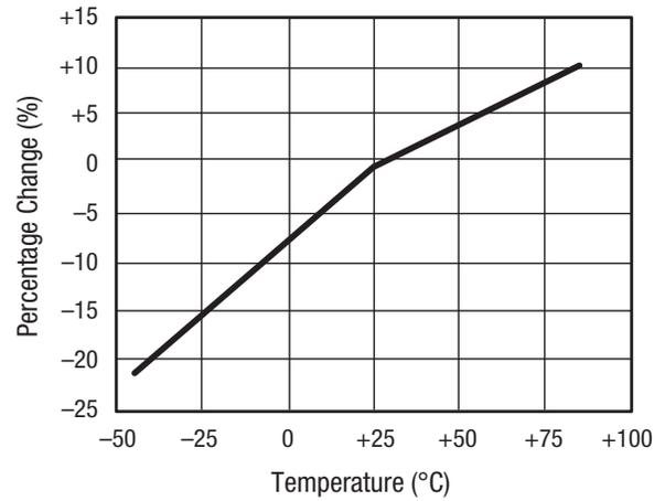
**Figure 2. Relative Series Resistance Change vs Temperature @ 500 MHz**
