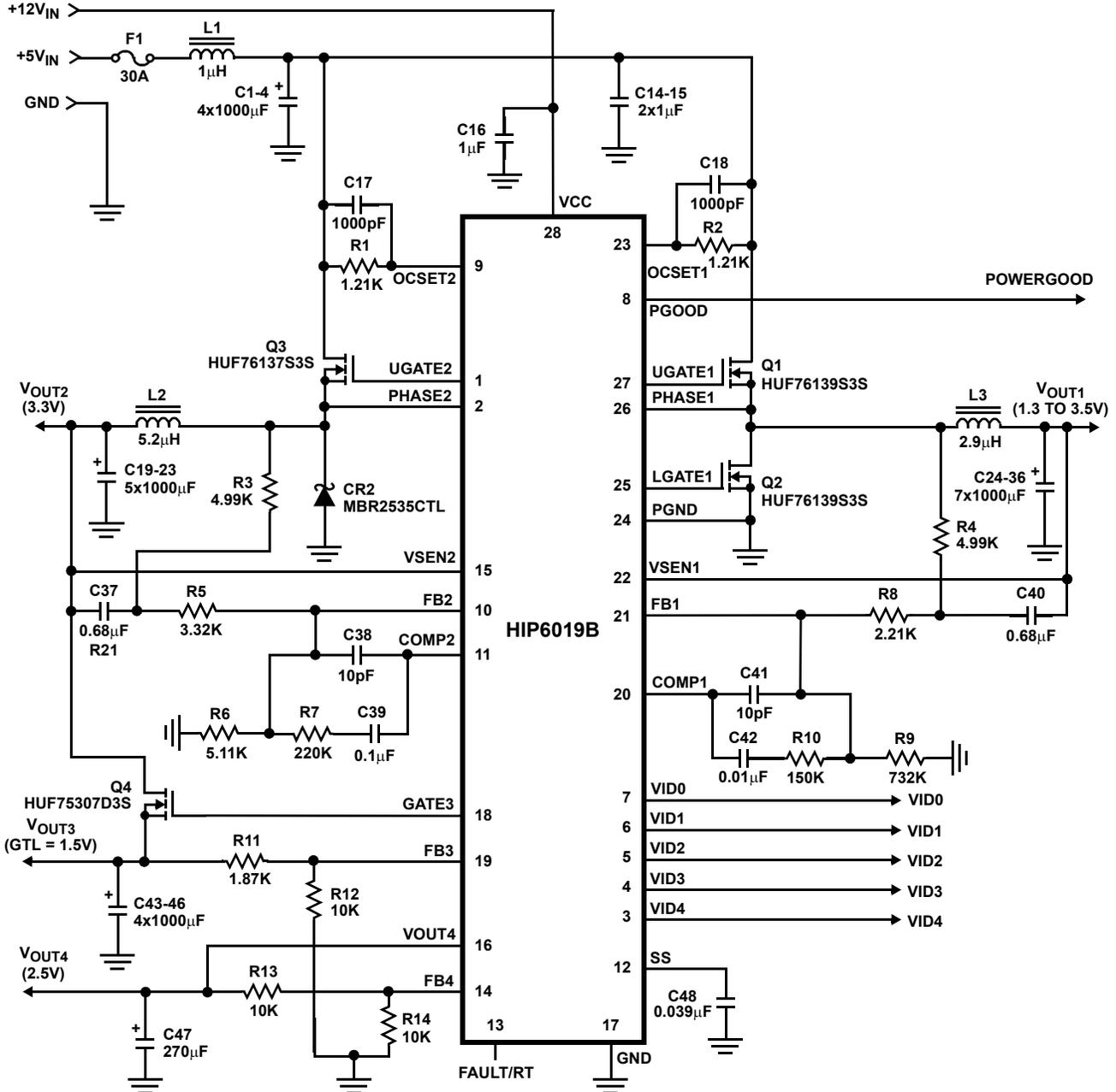
FIGURE 15. APPLICATION CIRCUIT
