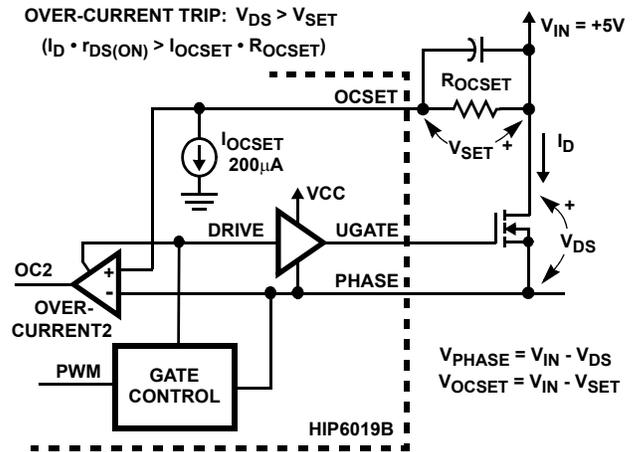
FIGURE 9. OVER-CURRENT DETECTION
