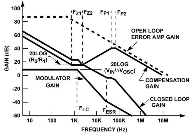
FIGURE 12. ASYMPTOTIC BODE PLOT OF CONVERTER GAIN
