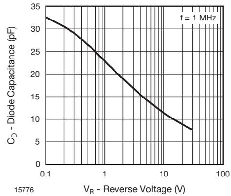
Fig. 6 - Typ. Diode Capacitance vs. Reverse Voltage
