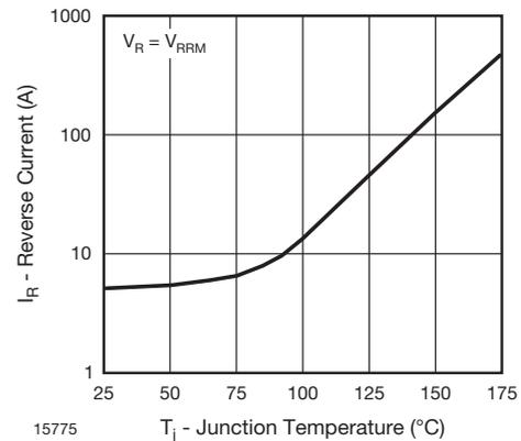
Fig. 3 - Max. Reverse Current vs. Junction Temperature
