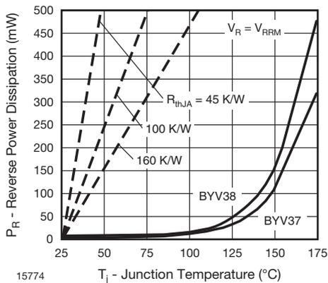
Fig. 2 - Max. Reverse Power Dissipation vs. Junction Temperature
