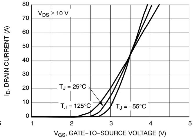
Figure 2. Transfer Characteristics
