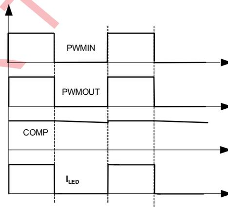
Figure 2—Fast and High Contrast Ratio PWM Dimming
