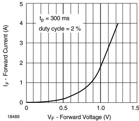
Fig. 2 - Typical High Current Forward Conduction Curve
