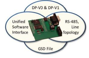
master at either DP-V0 or DP-V1 performance levels. DP-V0 supports basic cyclic data exchange, and DP-V1 supports both cyclic and acyclic data exchange. Several alarm types are supported as part of the acyclic data exchange. Data rates down to 1 ms are supported at the maximum I/O data size of 244 bytes.
