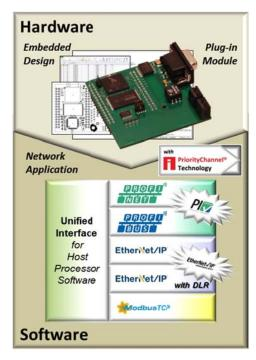
As an embedded design, the *Network Interface* hardware design can be integrated directly using the schematics provided. Also provided are the Bill of Materials and example layouts to minimize the hardware design effort. Software for the embedded design is provided as firmware that is downloaded to Flash. Whether using the *Network Interface* as a module or an embedded design, no software development is required and there are no license fees or royalties.
