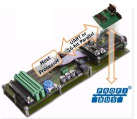
it is also easy to specify how parameters will be passed to the PROFIBUS controller using the GSD file. Since the Host is only passing parameters, the Host software does not have to change if PROFIBUS network parameters change or if another Industrial Ethernet protocol is used. Example C-code is provided to minimize the software effort for the Host / Network Interface communication.
