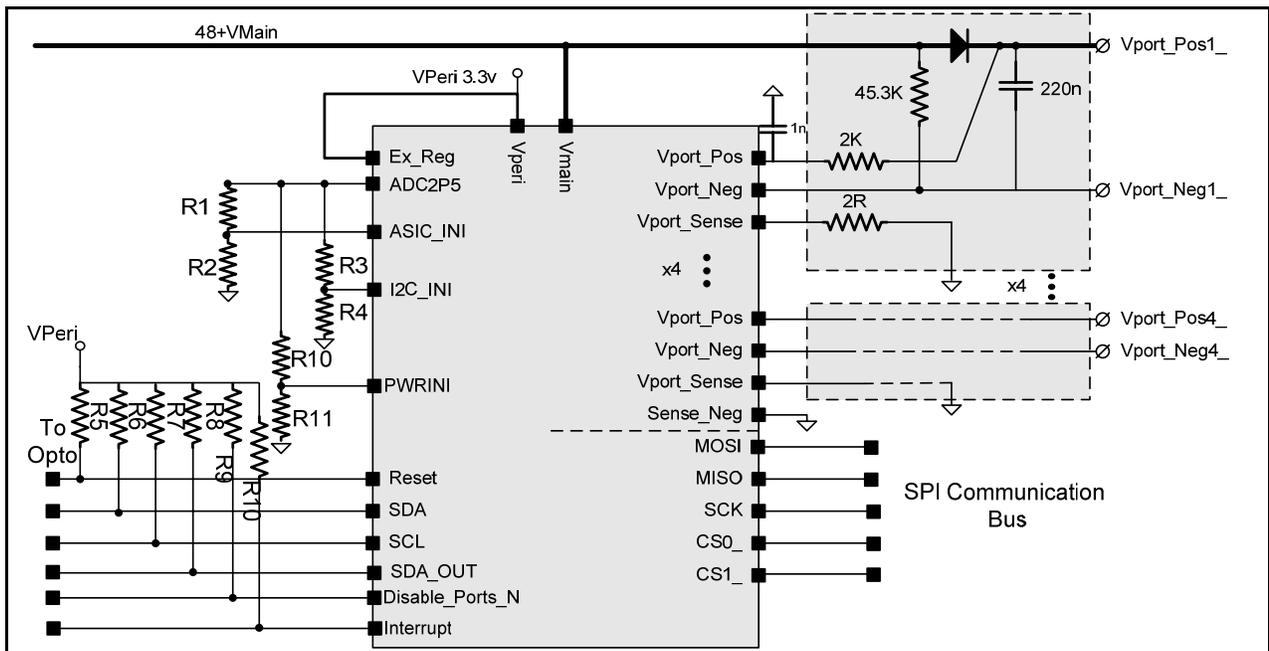
**Figure 4: Single-port Application with AC Disconnect Support**
