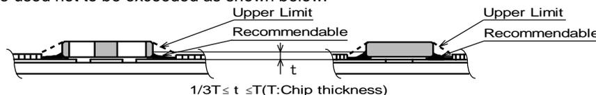
Accordingly increasing the solder volume, the mechanical stress to product is also increased. Excessive solder volume may cause the failure of mechanical or electrical performance.
