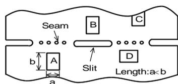
Products (A,B,C,D) shall be located carefully so that products are not subject to the mechanical stress due to warping the board. Because they may be subjected the mechanical stress in order of  $A > C > B \approx D$ .
