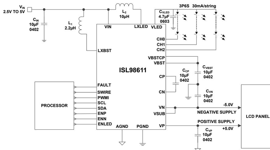
FIGURE 1. TYPICAL APPLICATION CIRCUIT FOR 3-CHANNEL LED DRIVER
