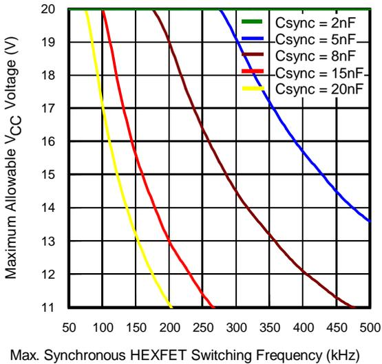
Fig 11. Max. V<sub>CC</sub> Voltage vs. Synchronous Rectifier Switching Freq, T<sub>J</sub>=125 C, T<sub>IC</sub> = 85 C, external R<sub>G</sub>=1Ω, 1Ω HEXFET Gate Resistance included
