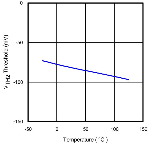
**Fig 4.** V<sub>TH2</sub> vs. Temp.
