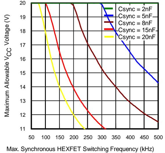
Fig 12. Max. V<sub>CC</sub> Voltage vs. Synchronous Rectifier Switching Freq, T<sub>J</sub>=125 C, T<sub>IC</sub> = 85 C, external R<sub>G</sub>=2Ω, 1Ω HEXFET Gate Resistance included
