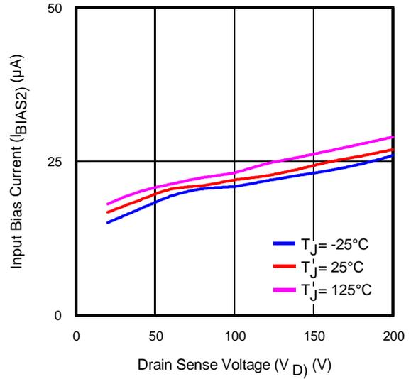
Fig 10. Input Bias Current vs. V<sub>D</sub>.
