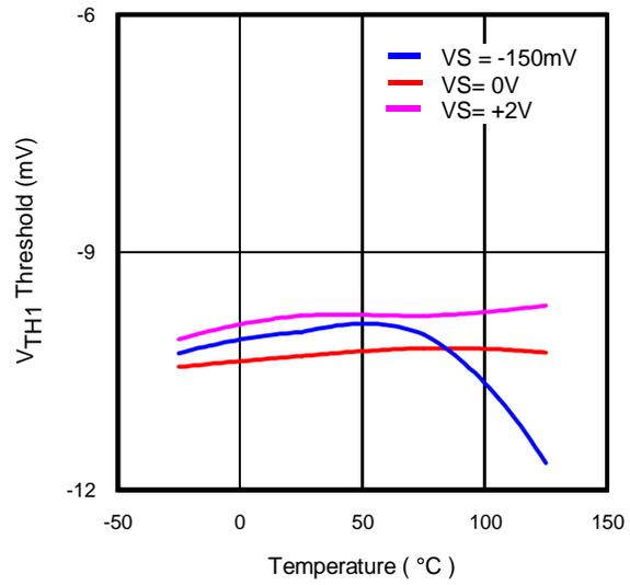
**Fig 6.**  $V_{TH1}$  vs. Temp. and Common Mode (OVT=Floating)
