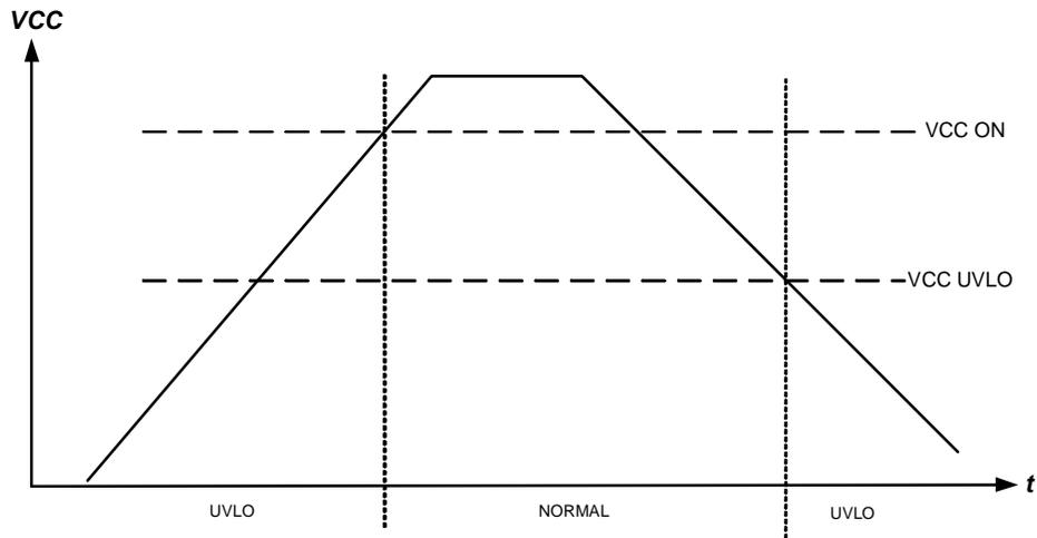
**Fig. 14 - V<sub>CC</sub> Under Voltage Lockout**
