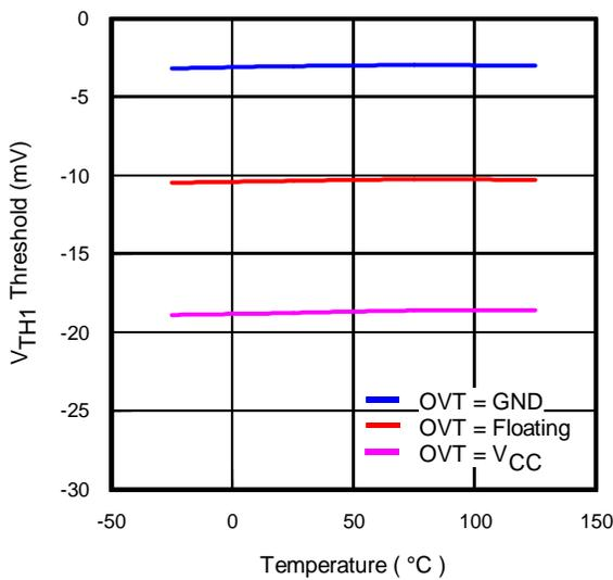
**Fig 3.** V<sub>TH1</sub> vs. Temp.
