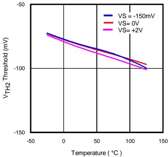
**Fig 7.**  $V_{TH2}$  vs. Temp. and Common Mode (OVT=GND)
