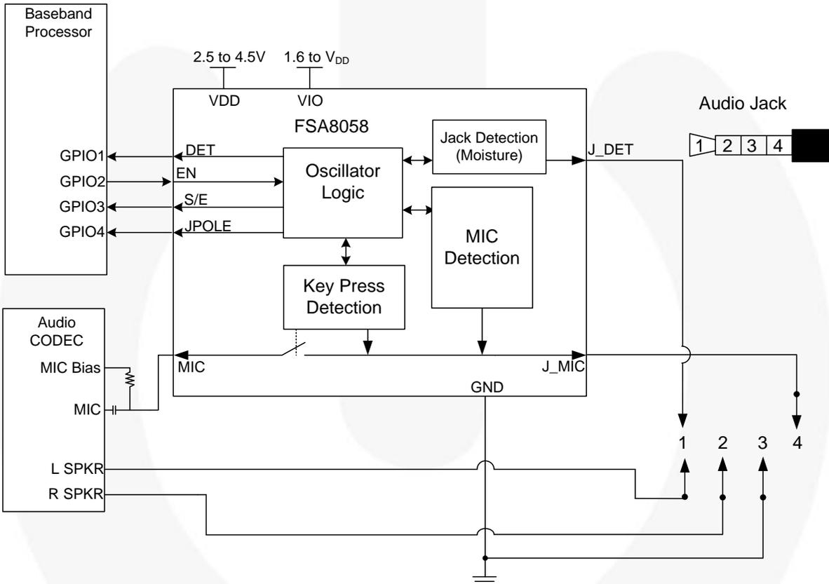
Figure 3. Typical Application Diagram
