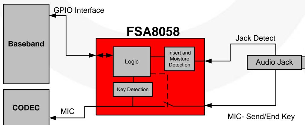
Figure 1. System Diagram
