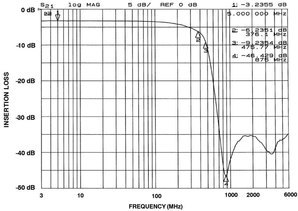
Figure 2. Insertion Loss vs. Frequency (2.5 V Bias)
