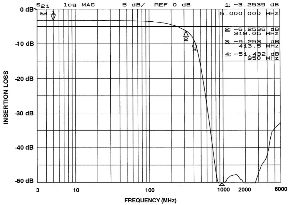
Figure 1. Insertion Loss vs. Frequency (0 V Bias)
