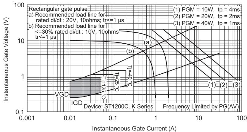
Fig. 11 - Gate Characteristics
