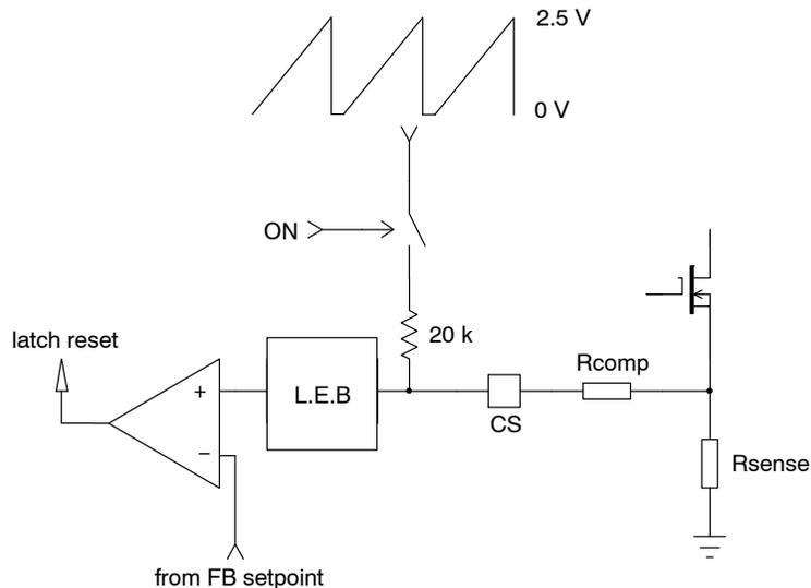
**Figure 41. Inserting a resistor in series with the current sense information brings slope compensation and stabilizes the converter in CCM operation.**
