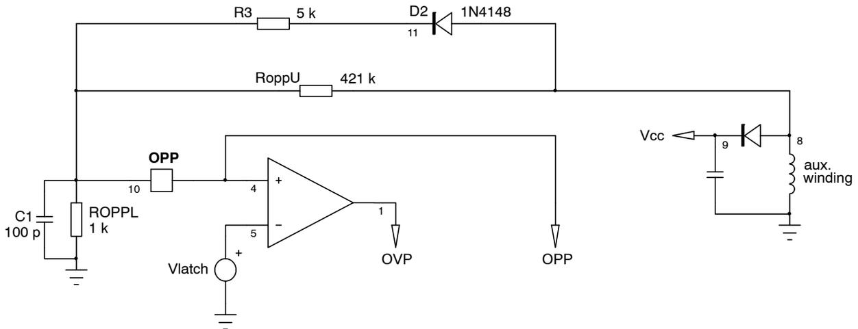
Figure 42. A simple resistive divider brings the OPP pin above 3 V in case of a  $V_{\text{cc}}$  voltage runaway above 18 V.
