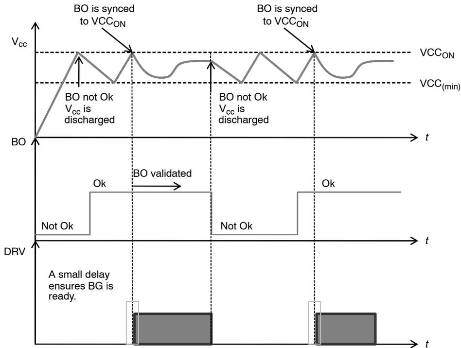
**Figure 52. The brown-out recovery is always synchronized to the  $V_{cc}$  signal: when it reaches  $V_{CCON}$ , the driver delivers the output pulses.**
