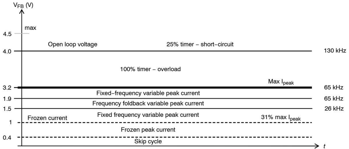
**Figure 48. Depending on the feedback level, the timer will take two different values: it will authorize a transient overload, but will reduce a short-circuit duration.**
