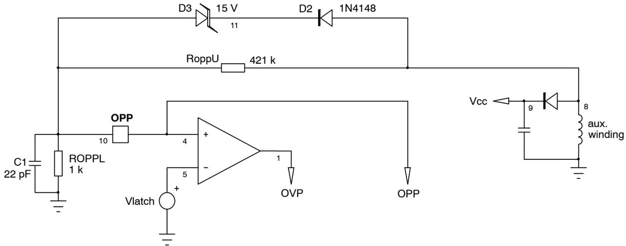
Figure 43. A Zener diode in series with a diode helps to improve the noise immunity of the system.
