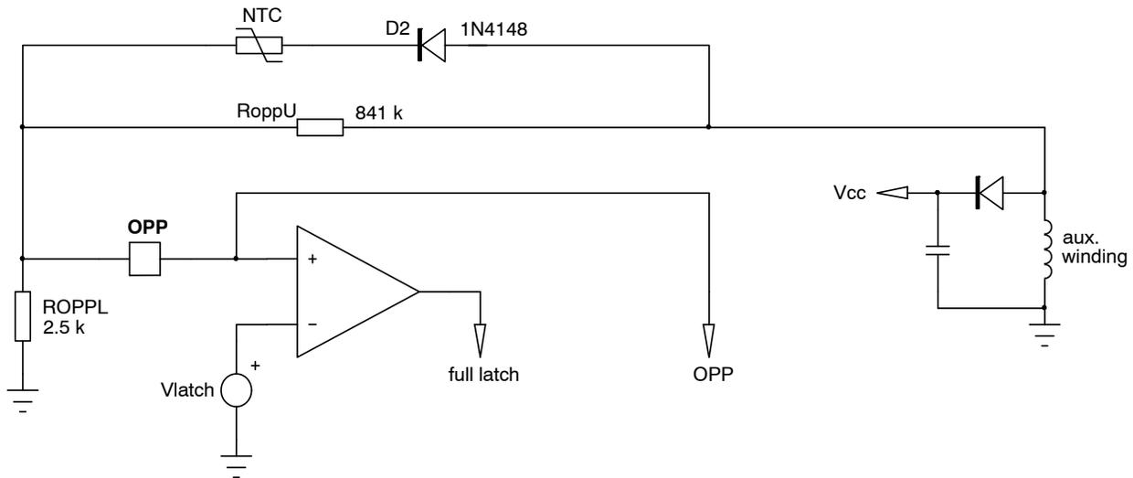
Figure 44. The internal circuitry hooked to pin 1 can be used to implement over temperature protection (OTP).
