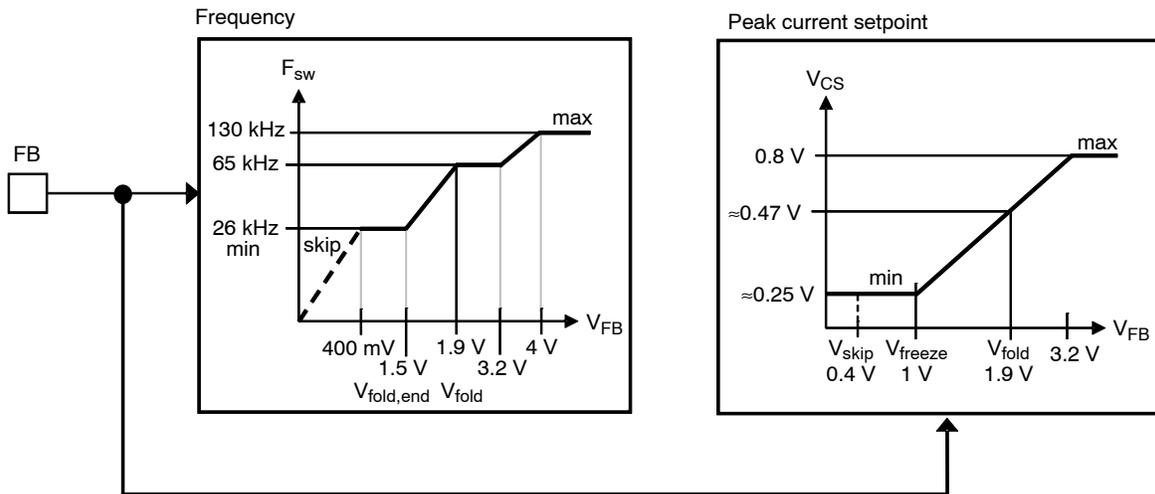
Figure 38. By observing the voltage on the feedback pin, the controller reduces its switching frequency for an improved performance at light load.
