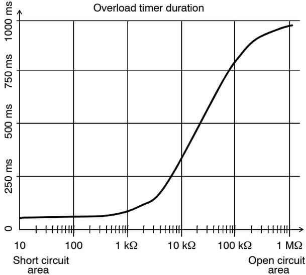
Figure 50. This curve shows how to program the OVL timer duration.
