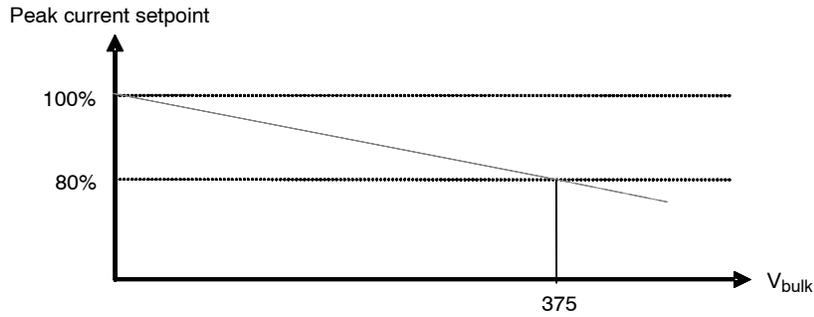
Figure 37. The peak current regularly reduces down to 20% at 375 V dc.
