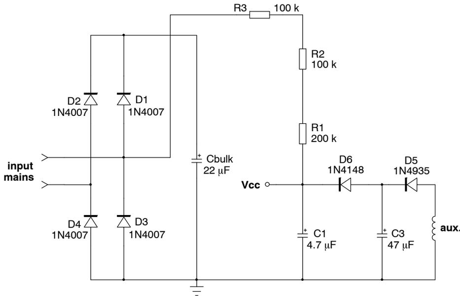
**Figure 33. The startup resistor can be connected to the input mains for further power dissipation reduction.**
