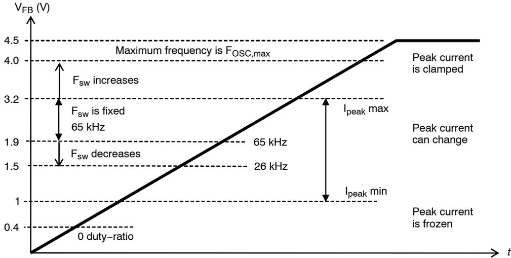
**Figure 47. The feedback pin modulates the frequency up to 130 kHz (short-circuit, maximum power) or down to 26 kHz in frequency foldback.**
