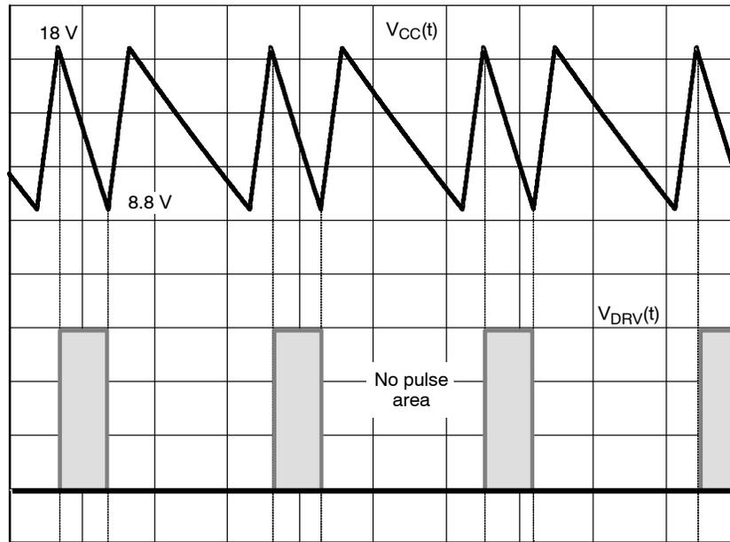
**Figure 39. An auto-recovery hiccup mode is entered in case a faulty event longer than 100 ms is acknowledged by the controller.**
