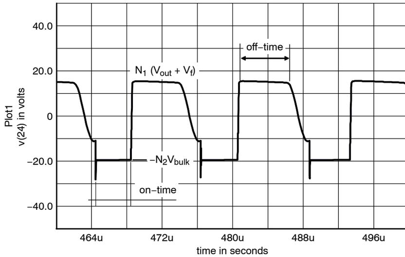
**Figure 35. The signal obtained on the auxiliary winding swings negative during the on-time.**
