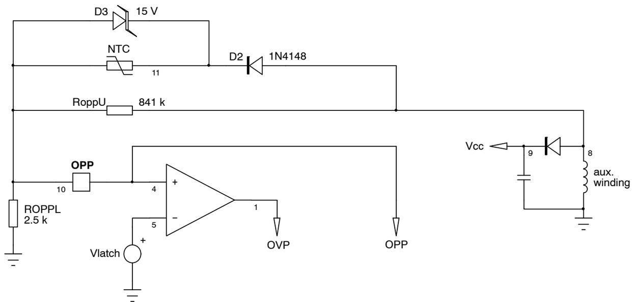
Figure 45. With the NTC back in place, the circuit nicely combines OVP, OTP and OPP on the same pin.
