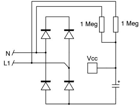
**Figure 34. The full-wave connection ensures latch current continuity as well as a X2-discharge path.**
