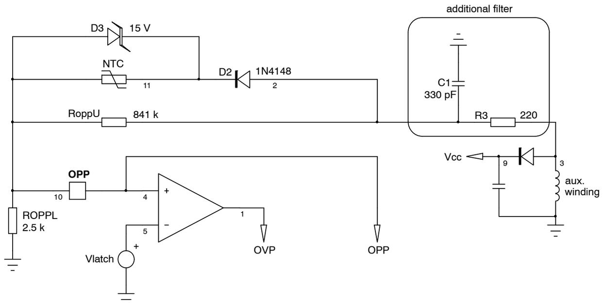
Figure 46. A small RC filter avoids the fast rising spikes from reaching the protection pin of the NCP125x in presence of energetic perturbations superimposed on the input line.
