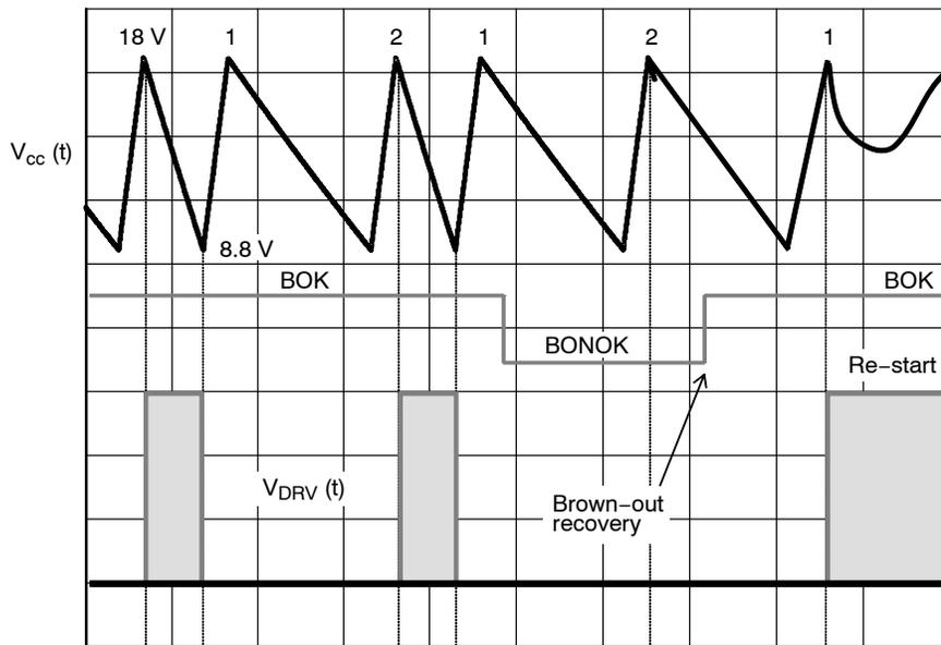
**Figure 40. The hiccup latch is reset when a brown-out transition is detected to shorten the re-start time.**
