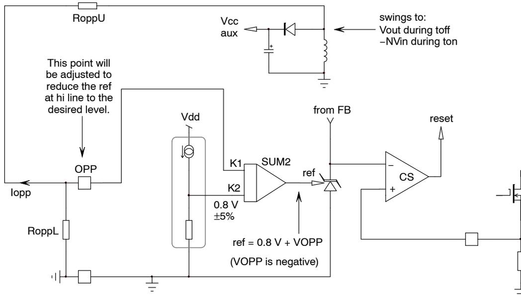
**Figure 36. The OPP circuitry affects the maximum peak current set point by summing a negative voltage to the internal voltage reference.**
