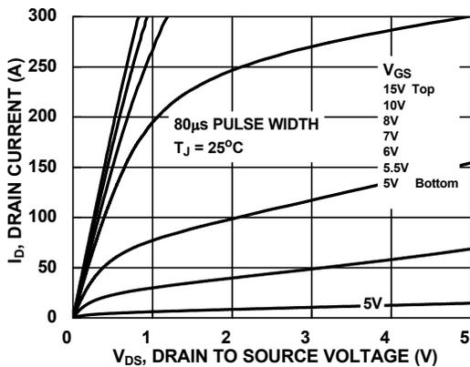
Figure 9. Saturation Characteristics
