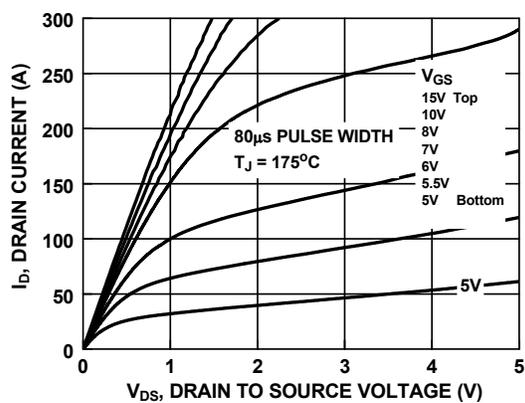
Figure 10. Saturation Characteristics
