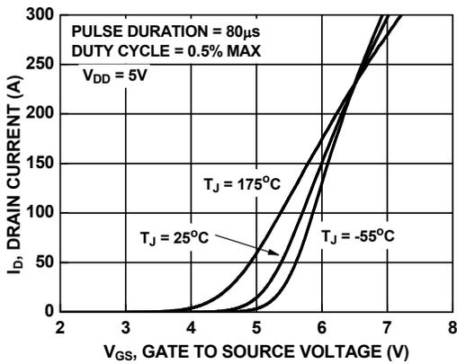
Figure 7. Transfer Characteristics
