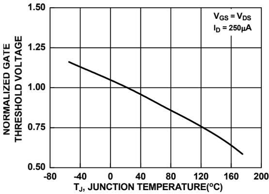
Figure 13. Normalized Gate Threshold Voltage vs. Temperature
