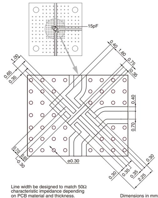
Line width be designed to match 50Ω characteristic impedance depending on PCB material and thickness.
