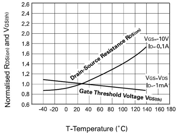
**Normalized  $R_{DS(on)}$  and  $V_{GS(th)}$  vs Temperature**
