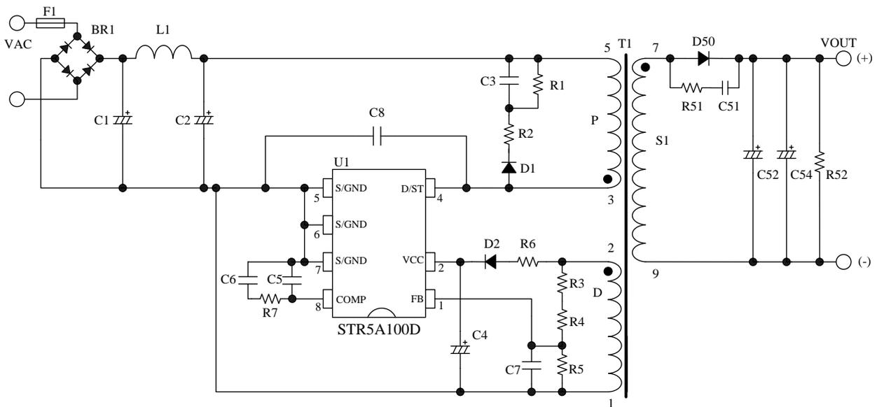
Figure 12-2 Circuit schematic for PCB circuit trace layout
