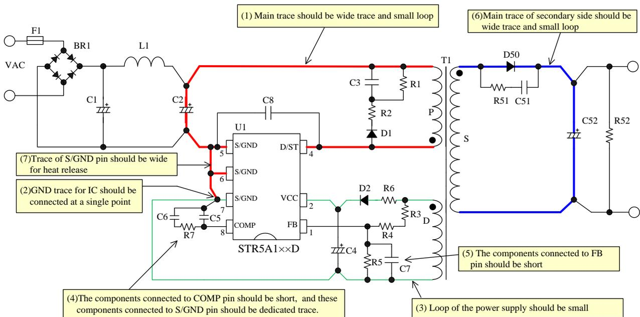
Figure 11-7 Example of peripheral circuit around the IC
