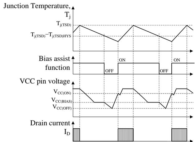
Figure 10-13 TSD operational waveforms
