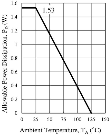
Figure 4-3 Ambient Temperature versus Power Dissipation Curve
