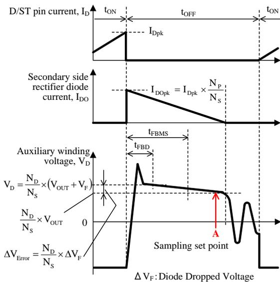
Figure 10-6 Detection timing of auxiliary winding voltage
