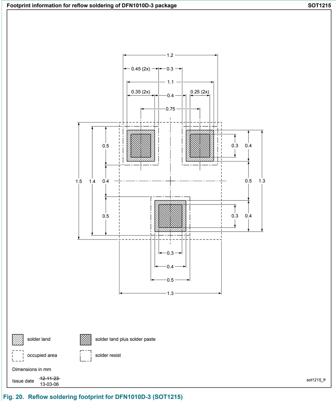
Fig. 20. Reflow soldering footprint for DFN1010D-3 (SOT1215)
