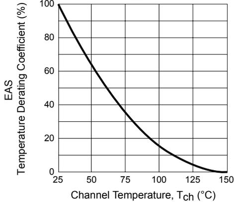
MOSFET Temperature versus Power Dissipation Curve
