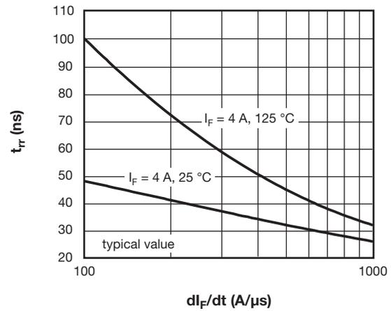
Fig. 6 - Typical Reverse Recovery vs.  $di_F/dt$
