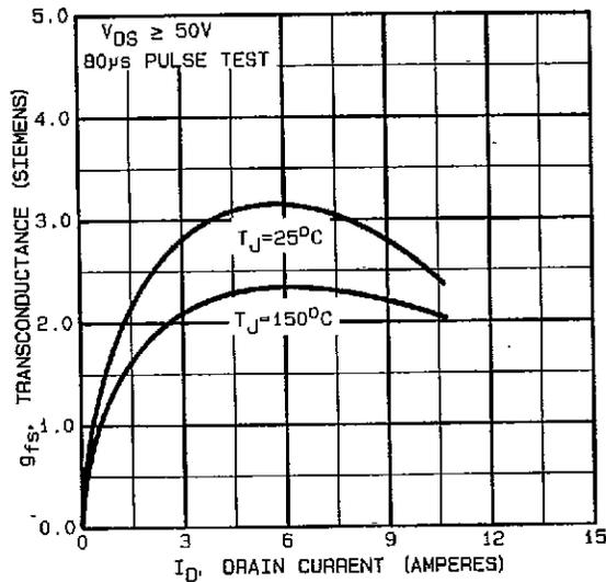
Fig. 12c - Typical Transconductance vs. Drain Current
