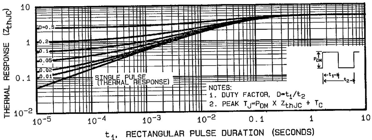
Fig. 11 - Maximum Effective Transient Thermal Impedance, Junction-to-Case
