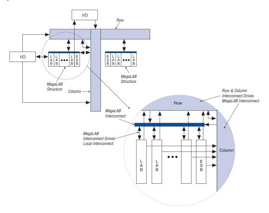
Figure 10. FastTrack Connection to Local Interconnect
