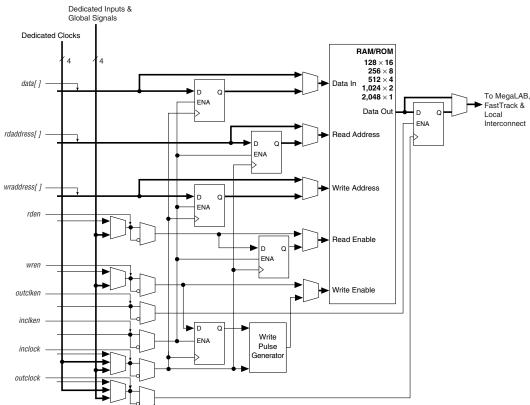
Figure 21. ESB in Input/Output Clock Mode Note (1)
