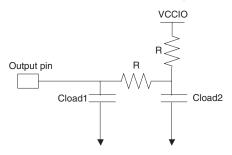
Figure 38. AC Test Conditions for the LVDS I/O Standard
