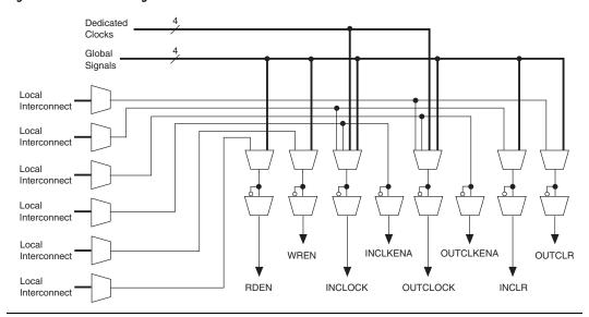
An ESB is fed by the local interconnect, which is driven by adjacent LEs (for high-speed connection to the ESB) or the MegaLAB interconnect. The ESB can drive the local, MegaLAB, or FastTrack interconnect routing structure to drive LEs and IOEs in the same MegaLAB structure or anywhere in the device.
