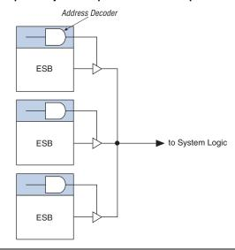
Figure 18. Deep Memory Block Implemented with Multiple ESBs
