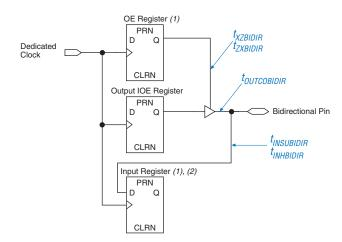
Figure 35. Synchronous Bidirectional Pin External Timing
