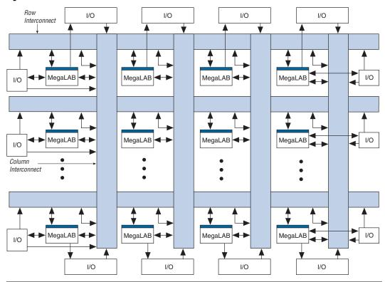
Figure 9. APEX 20KC Interconnect Structure
