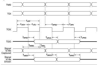
Figure 30. APEX 20KC JTAG Waveforms
