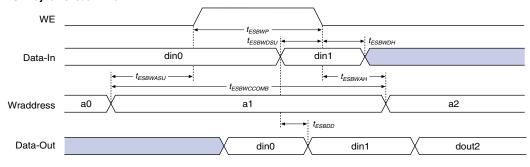
Figure 34. ESB Synchronous Timing Waveforms
