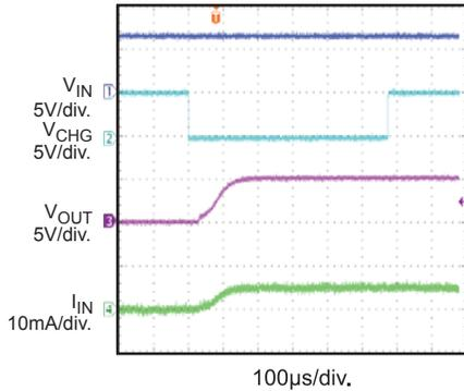
**Shut Down Low vs. Battery Charge**
