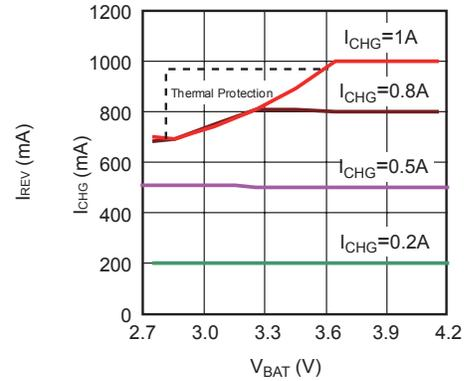
**Charge Current vs Input Voltage**
