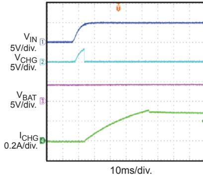
**Power Ramp Down vs. Battery Charge**
