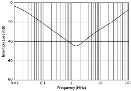
Common Mode Insertion Loss (Typ.)
