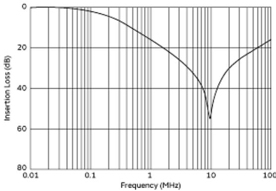
Differential Mode Insertion Loss (Typ.)
