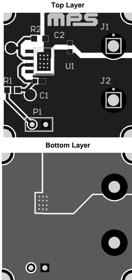
The  $V_{DD}$  decoupling capacitor should be closed to  $V_{DD}$  and A pins (C1 in the upper figure). The  $V_D$  resistor (R2 in the upper figure) connects a joint close to K pin and keeps the  $V_D$  trace short. MP6914DN-00A is a good example.
