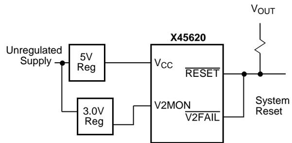
**Notice:** No external components required to monitor two voltages.
