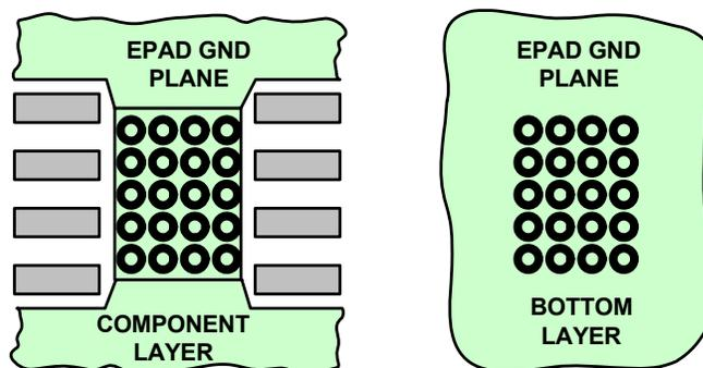
FIGURE 21. TYPICAL PCB PATTERN FOR THERMAL VIAS
