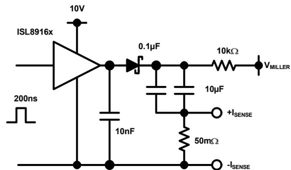
FIGURE 6. MILLER PLATEAU SOURCE CURRENT TEST CIRCUIT
