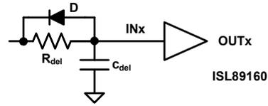
FIGURE 19. SETTING DELAYS WITH A RCD NETWORK
