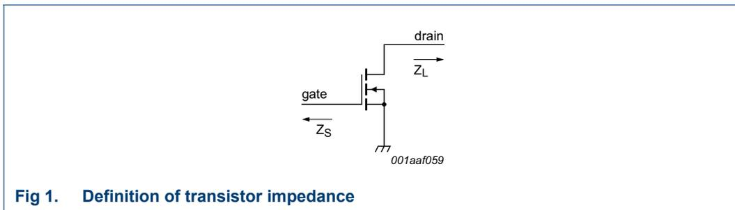
Fig 1. Definition of transistor impedance
