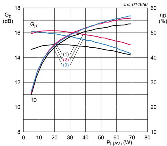
$V_{DS} = 28\text{ V}$ ;  $I_{Dq} = 250\text{ mA}$  (main device);  $V_{GS(amp)peak} = 0.7\text{ V}$ .
