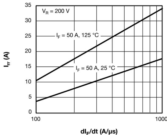
Fig. 9 - Typical  $I_{rr}$  Diode vs.  $di_F/dt$
