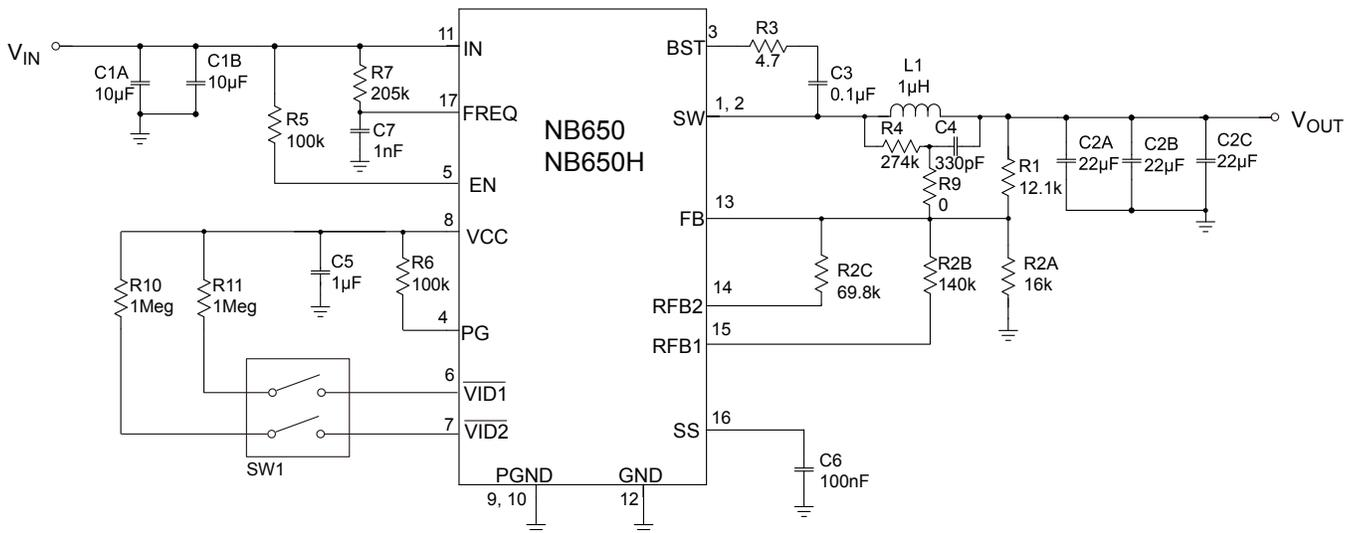
**Figure 13: Typical Application with Low-ESR Ceramic Capacitor**
