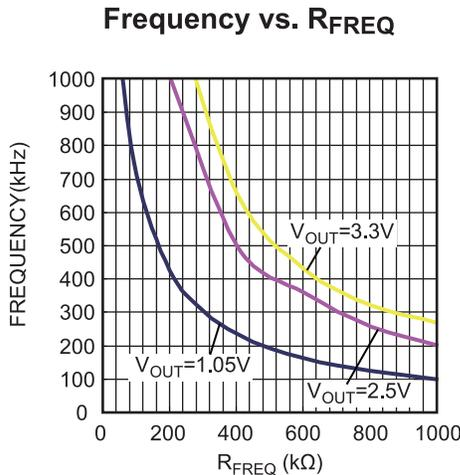
**Figure 4: Plot of V<sub>OUT</sub> as a Function of R<sub>FREQ</sub> and the Frequency**
