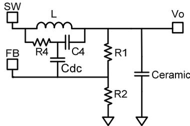
**Figure 11: Simplified Circuit with Ceramic DC-Blocking Capacitor**
