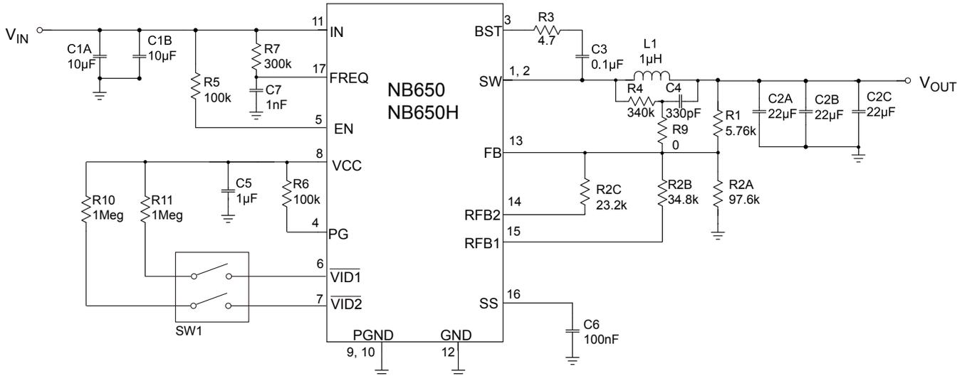
**Figure 15: Typical Application Circuit**
