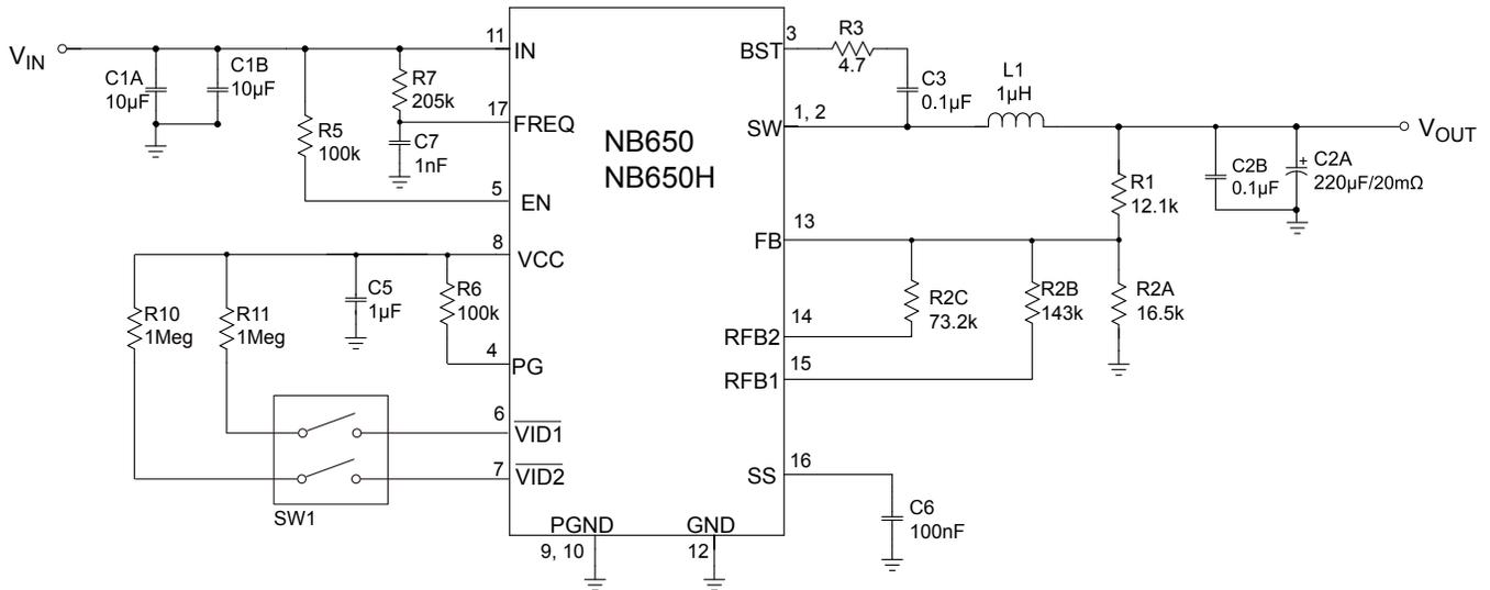
**Figure 12: Typical Application Circuit with No External Ramp**
