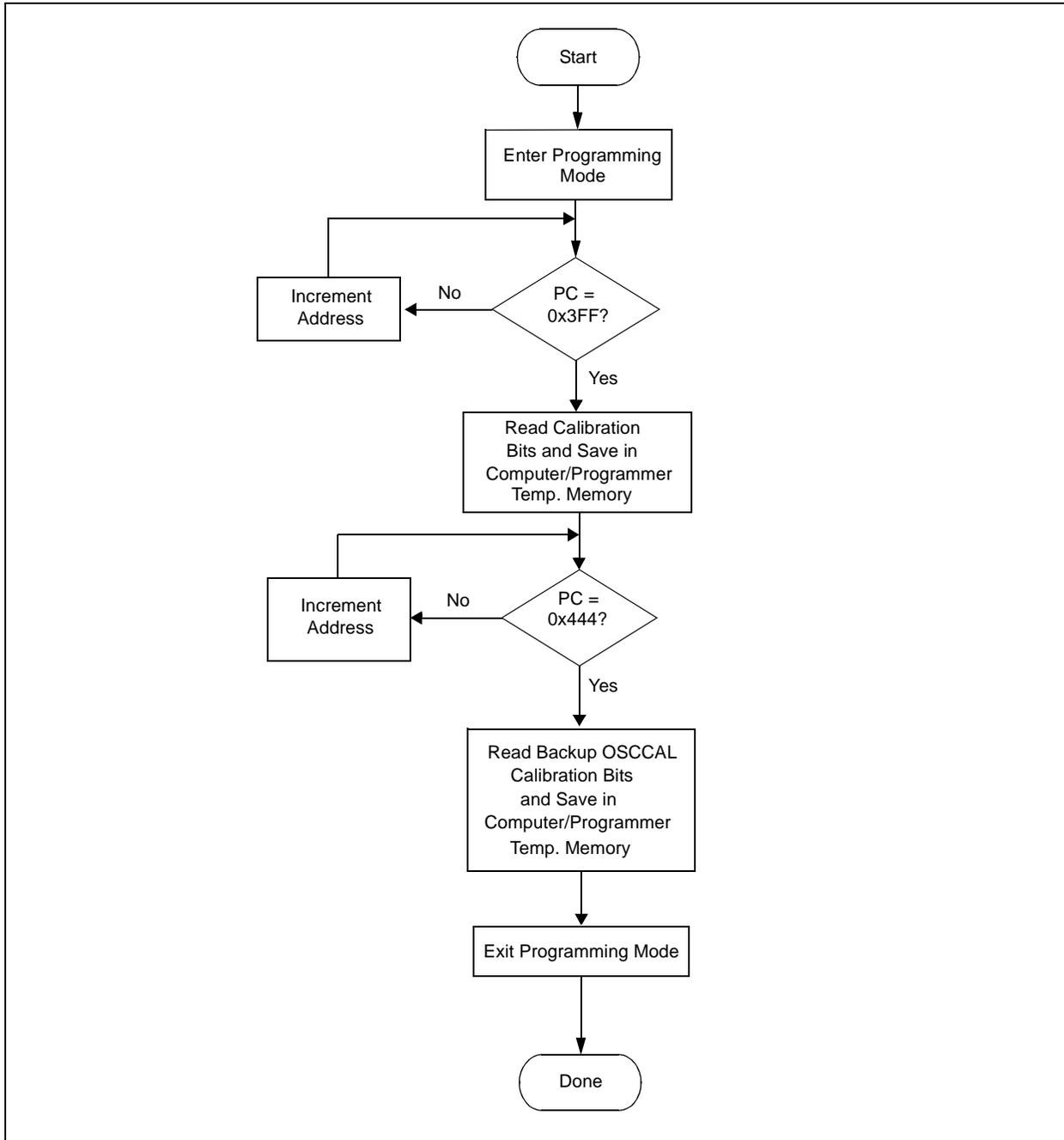
**FIGURE 3-9: RESTORING/PROGRAMMING THE OSCCAL CALIBRATION BITS**
