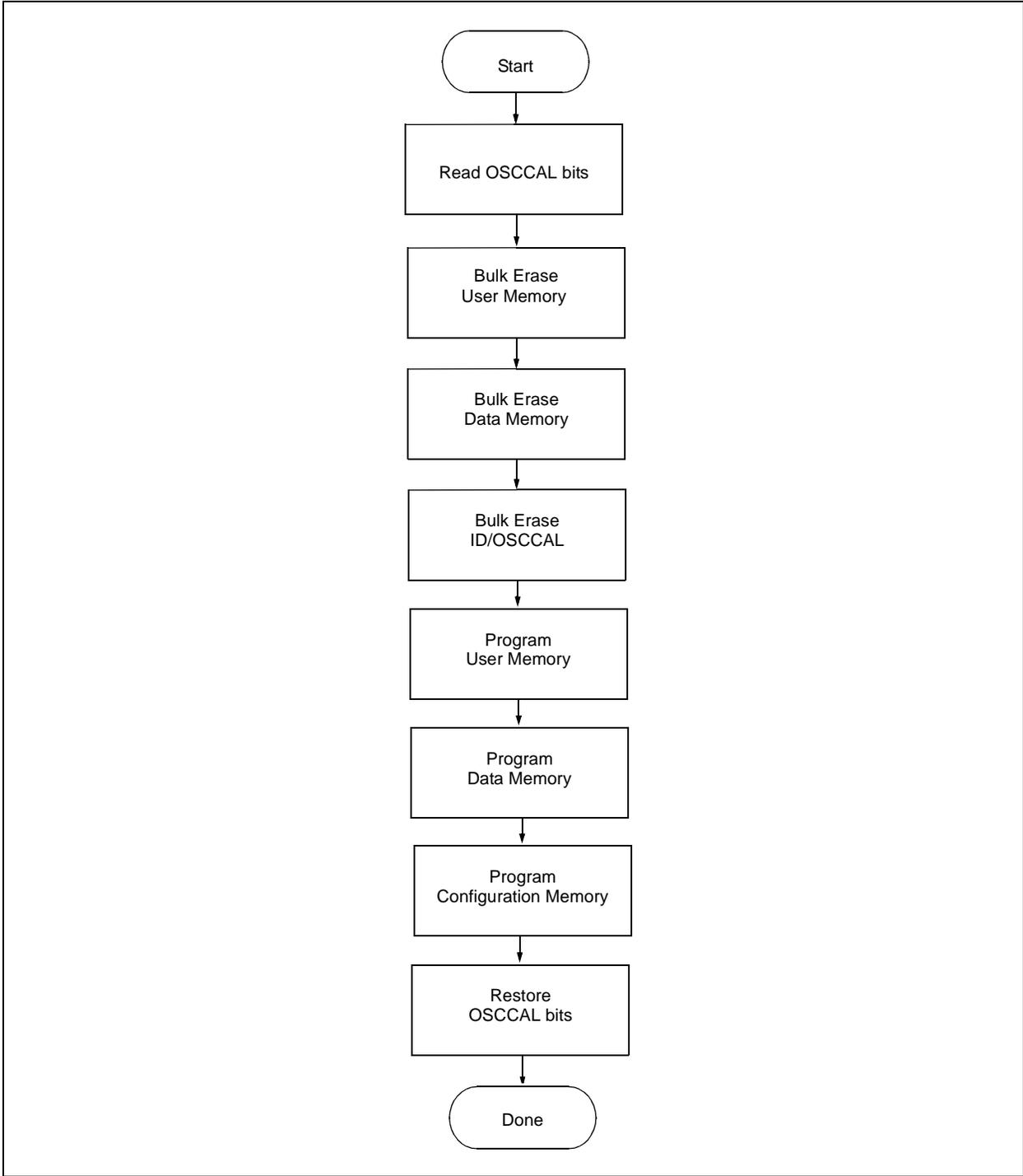
FIGURE 3-17: PROGRAM FLOWCHART – HIGH-LEVEL FULL DEVICE ERASE
