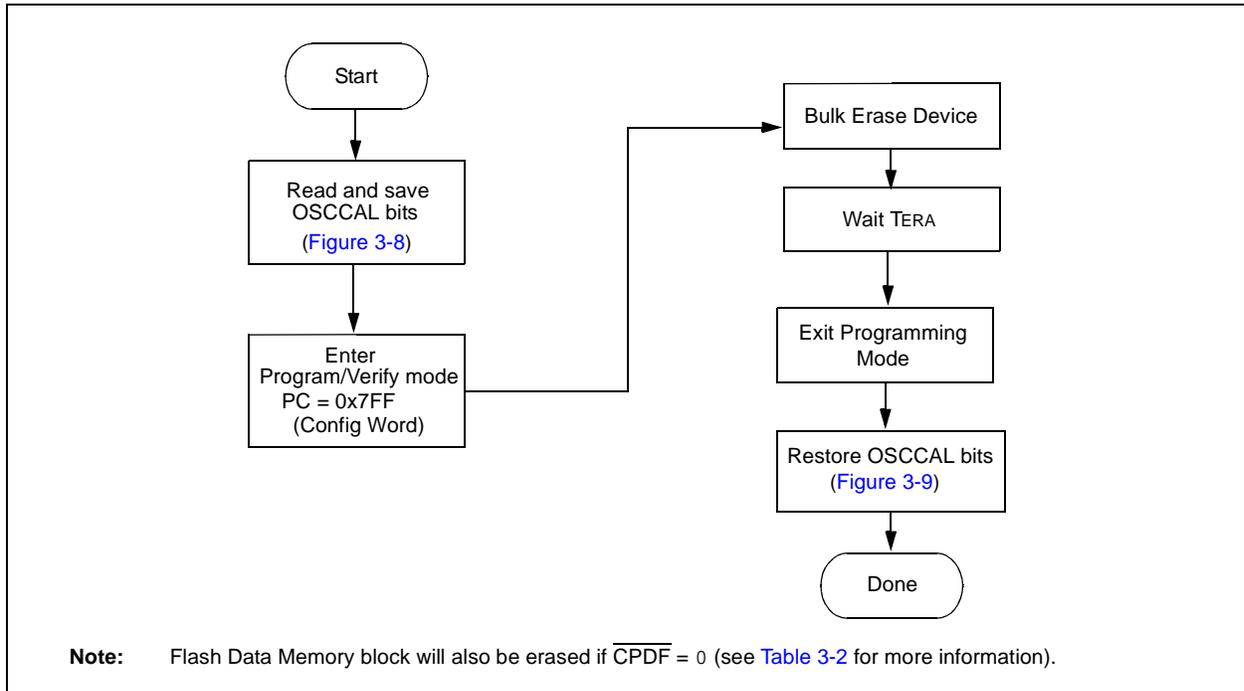
**FIGURE 3-14: PROGRAM FLOWCHART – ERASE FLASH DATA MEMORY**
