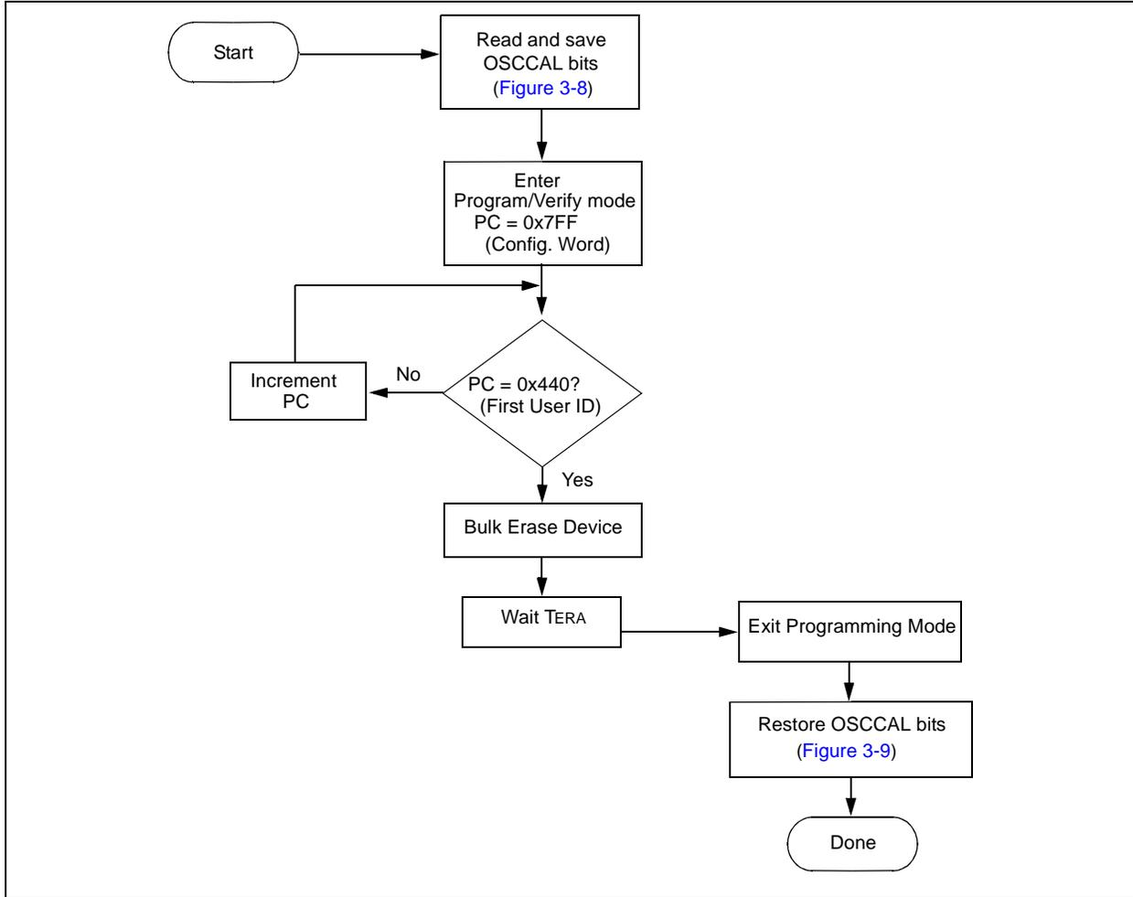
FIGURE 3-16: PROGRAM FLOWCHART – HIGH-LEVEL FULL DEVICE PROGRAM
