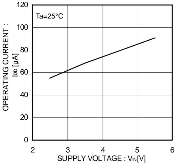
Figure 4. Operating current EN,/EN Enable
