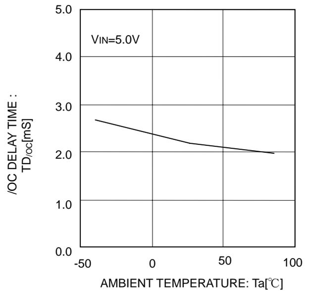
Figure 15. /OC output delay time
