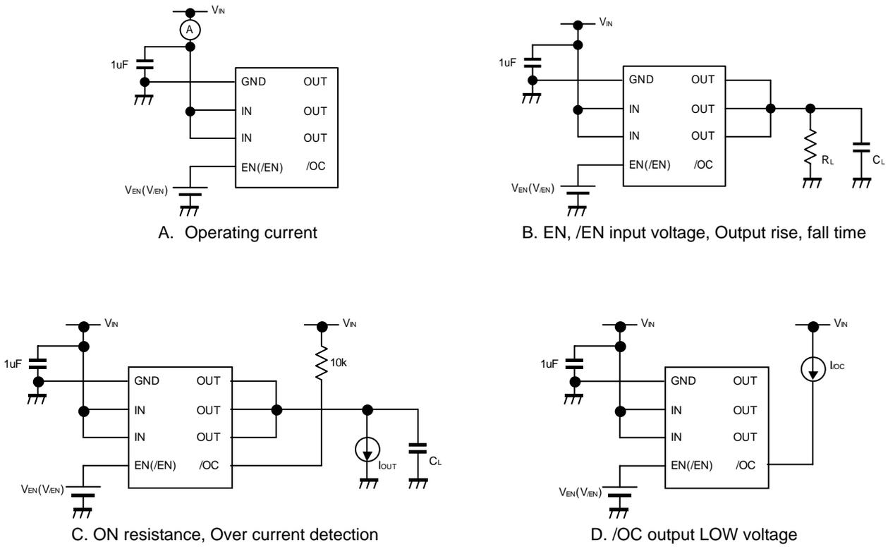
Figure 1. Measurement circuit
