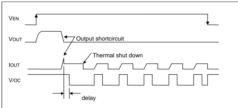
Figure 39. Over current detection, thermal shutdown timing (BD2065AFJ)
