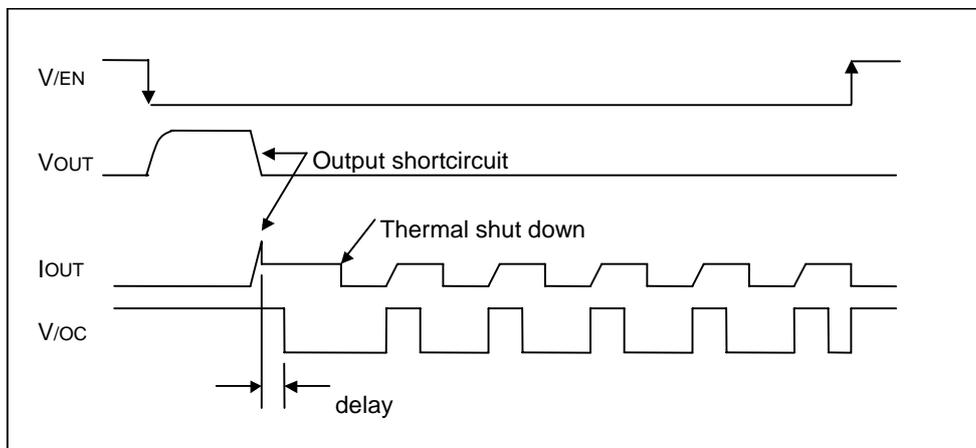
Figure 38. Over current detection, thermal shutdown timing (BD2061FJ)
