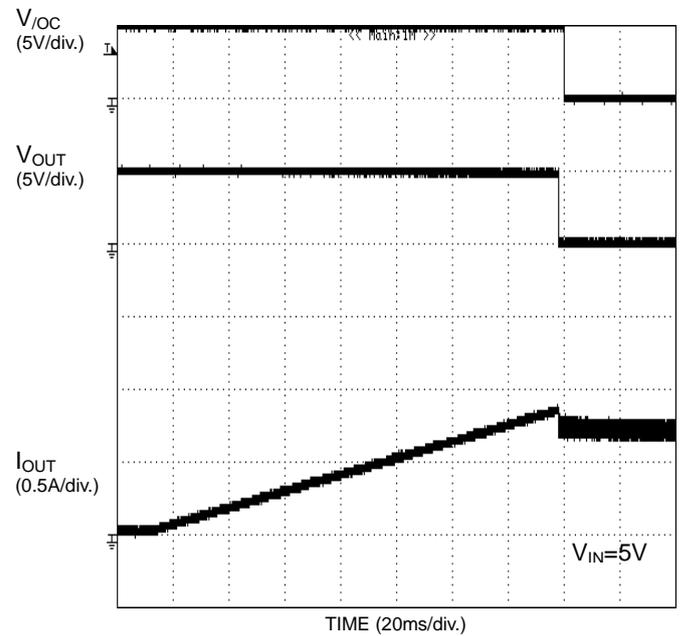
Figure 31. Over current response Ramped load (BD2061AFJ)
