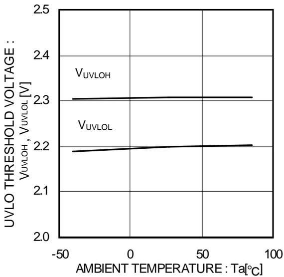
Figure 26. UVLO threshold voltage
