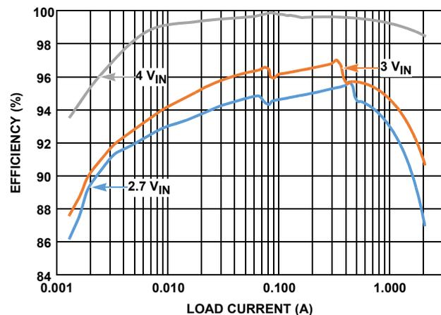
FIGURE 2. EFFICIENCY vs LOAD CURRENT,  $V_{OUT} = 3.3V$
