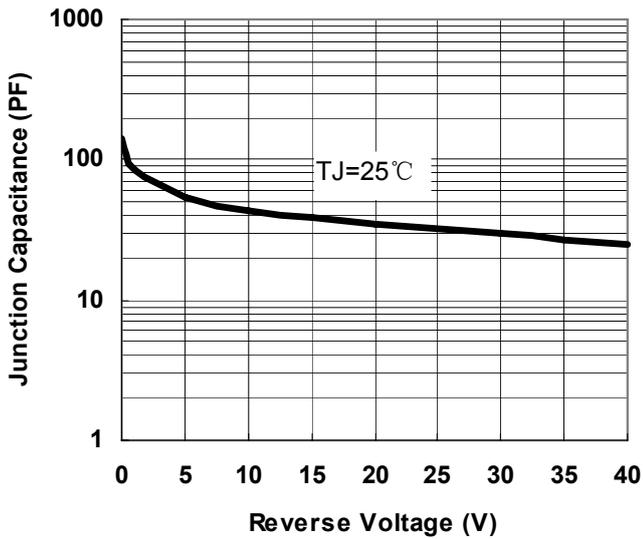
Fig.1-Typical Junction Capacitance
