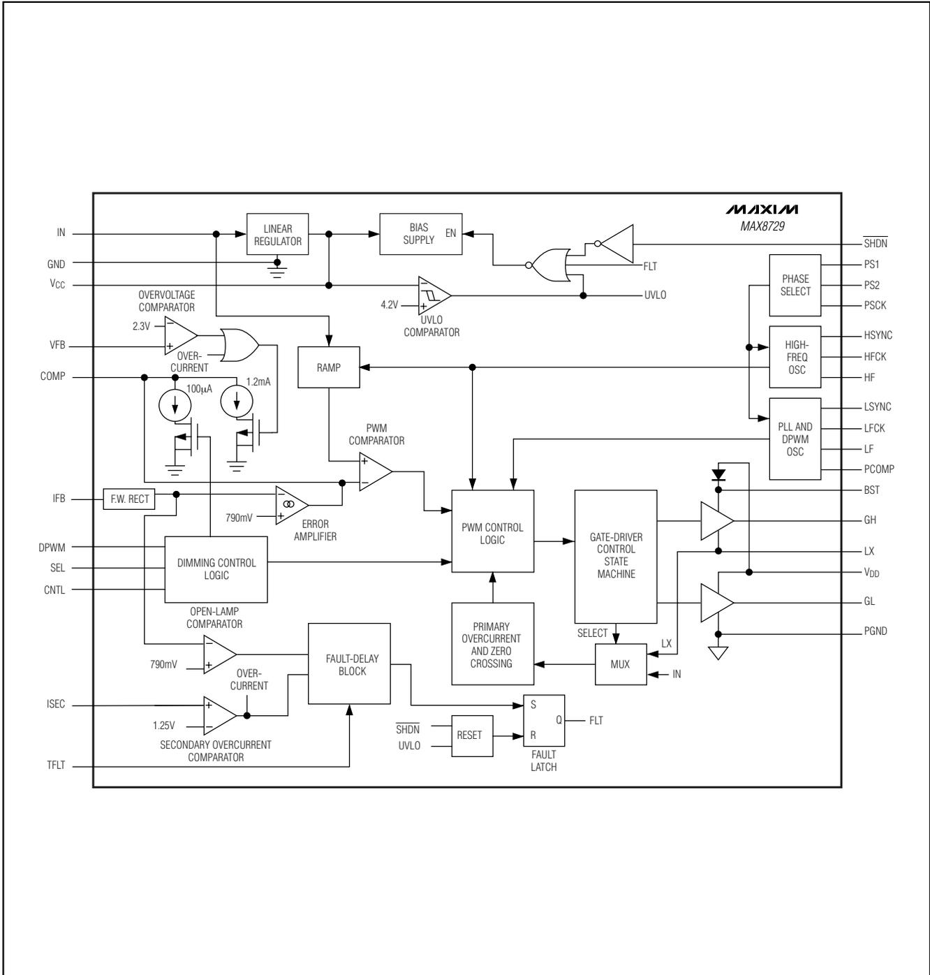
Figure 2. Functional Diagram
