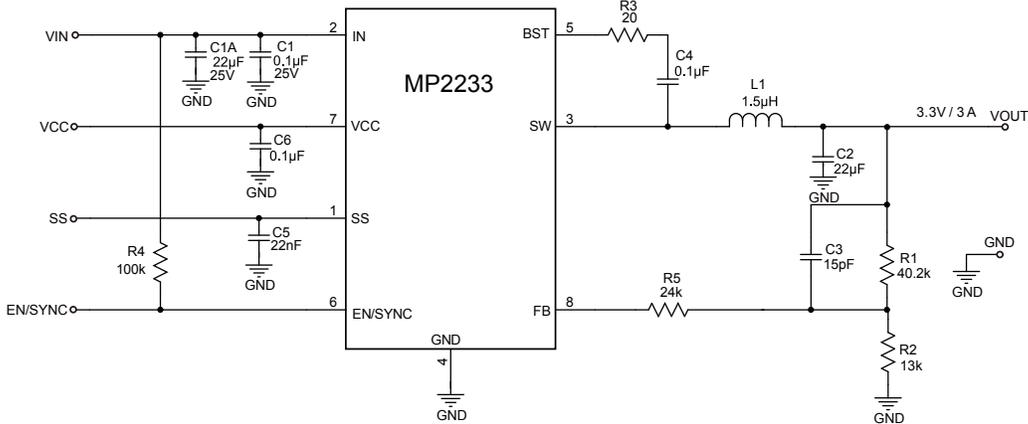
**Figure 8:  $V_{IN} = 12V$ , 3.3V/3A Output**
