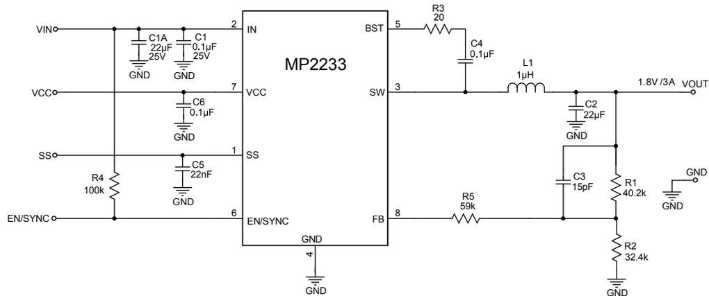
**Figure 10:  $V_{IN} = 12V$ , 1.8V/3A Output**
