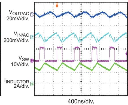
**Load Transient Reponse**  $I_{OUT} = 1.5A-3A$
