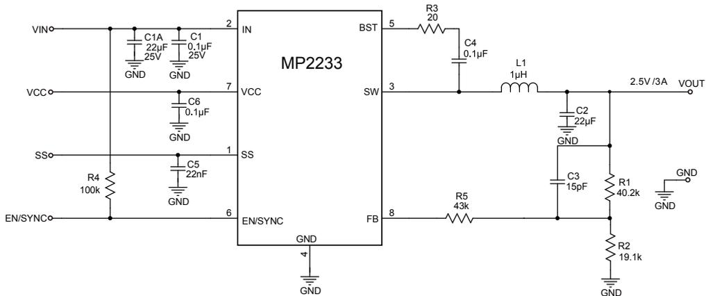
**Figure 9:  $V_{IN} = 12V$ , 2.5V/3A Output**
