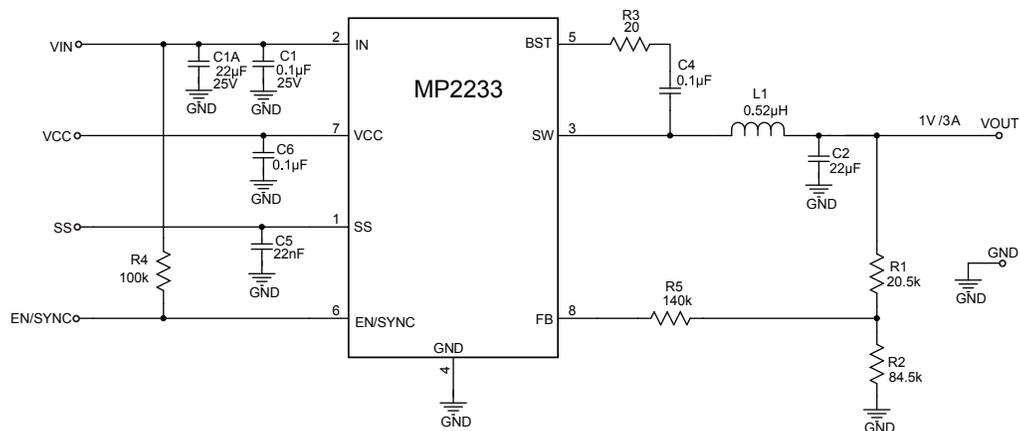
**Figure 12:  $V_{IN} = 12V$ , 1V/3A Output**
