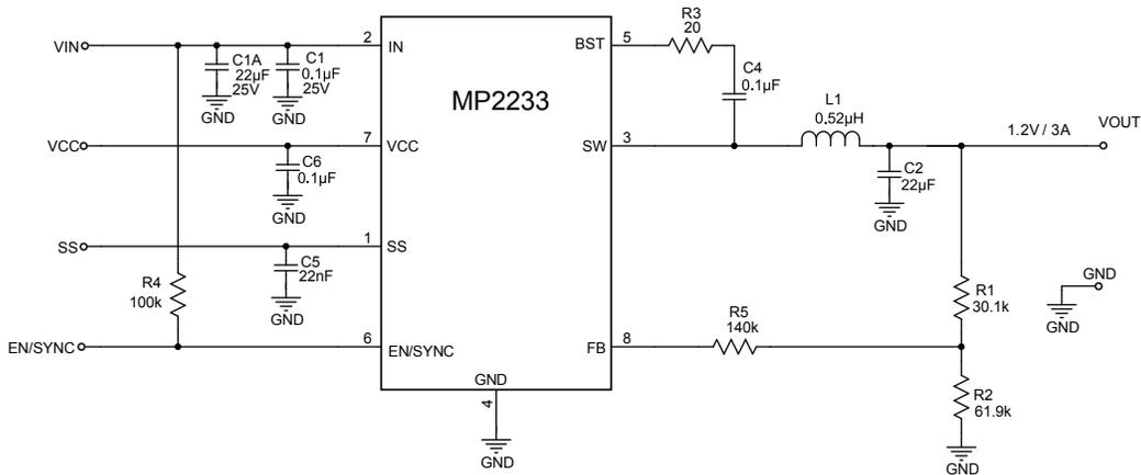
**Figure 11:  $V_{IN} = 12V$ , 1.2V/3A Output**
