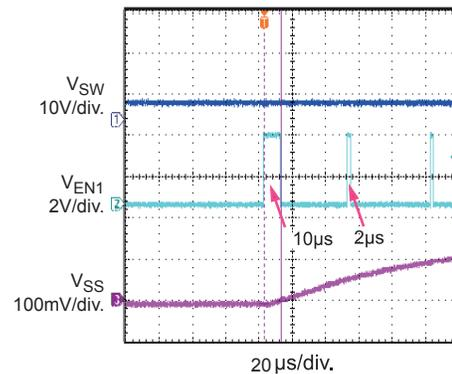
When MP1529 starts up under PWM Dimming mode, the first pulse width of EN1 is required to be more than 8μs to wake up the part. The pulse width can be as low as 2μs after MP1529 is active.
