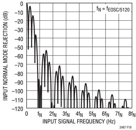
Figure 19. Input Normal Mode Rejection at DC
