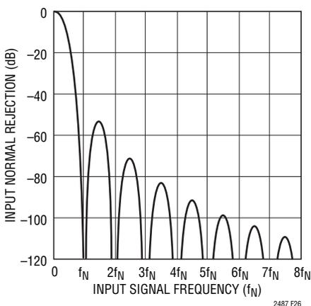
Figure 26. Input Normal Mode Rejection 2x Speed Mode
