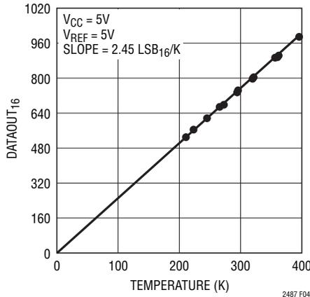
Figure 4. Internal PTAT Digital Output vs Temperature
