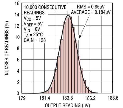
**RMS Noise vs  $V_{REF}$  (2x Speed Mode)**
