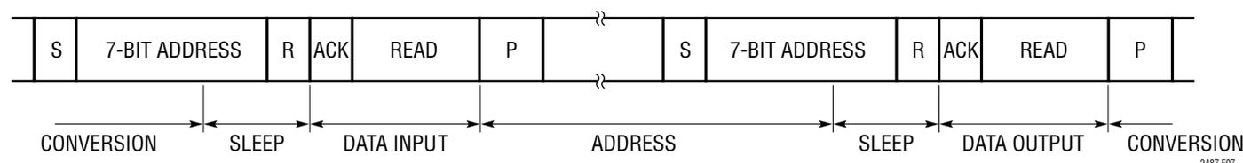
**Figure 7. Consecutive Reading with the Same Input/Configuration**
