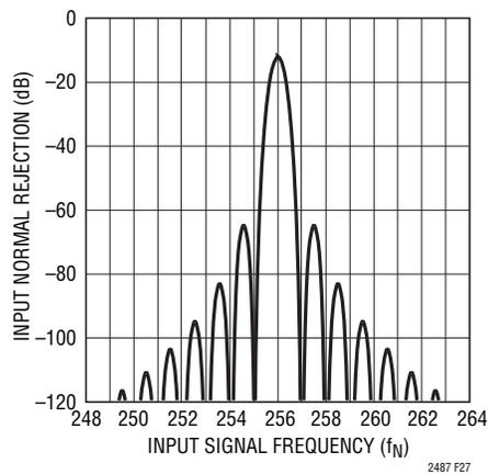
Figure 27. Input Normal Mode Rejection 2x Speed Mode
