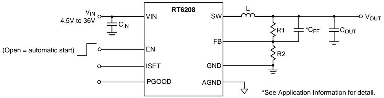
**(Recommended Component Selections for a 100mA Loading application of Popular output Voltage)**
