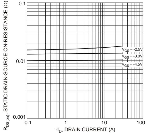
Fig. 4 On-Resistance vs. Drain Current and Gate Voltage
