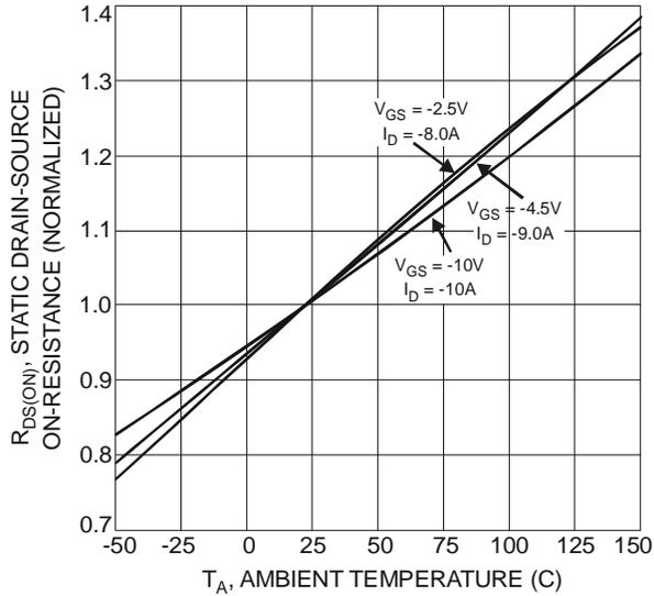
Fig. 3 Normalized Static Drain-Source On-Resistance vs. Ambient Temperature
