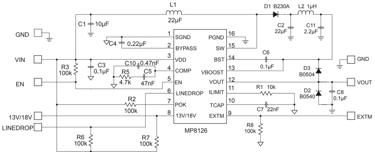
**Figure 4: Detailed Application Schematic**
