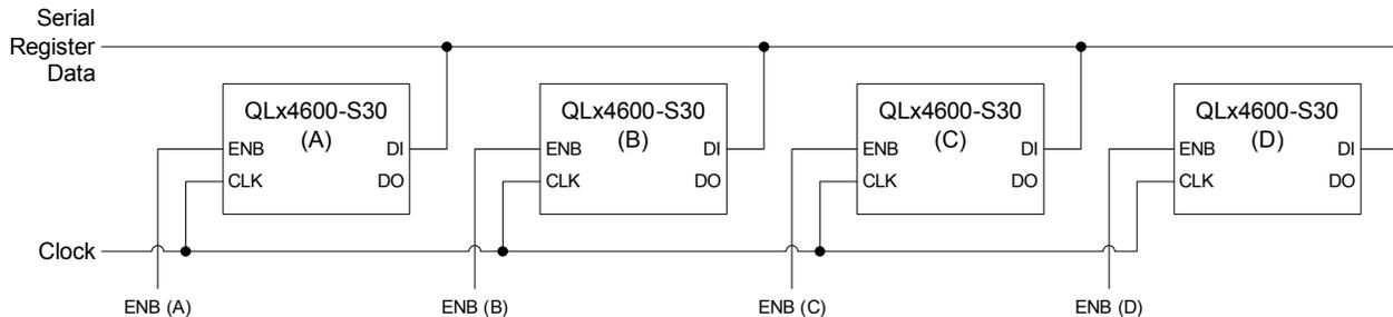
**FIGURE 29. SERIAL BUS PROGRAMMING MULTIPLE QLX4600-S30 DEVICES USING SEPARATE ENB SIGNALS**
