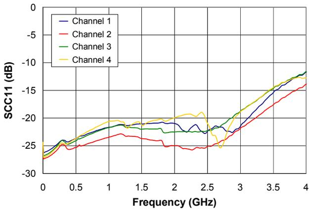
FIGURE 17. INPUT COMMON-MODE RETURN LOSS
